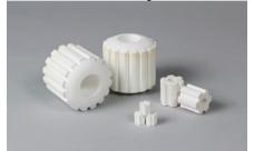
Christy's CATA-COGS™ are specialty hold down and support media which can dramatically reduce pressure drop in reactors such as Water Shift Converters due to their significantly increased void fraction when compared to ceramic or alumina balls. CATA-COGS™ are available in both our 99% alumina and ceramic formulations.
