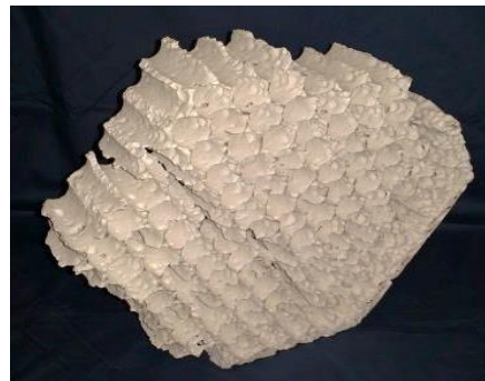
HT-LC Hexagonal Tile & PROX-SVERS® Corroded HT-99 Hexagonal Tile (99% Al 2 O 3 )
